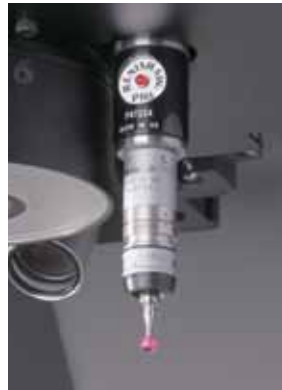
Renishaw® TP20 Touch Trigger Probing system
