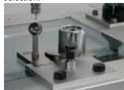
Calibration sphere and ring gauge set included in the basic set
