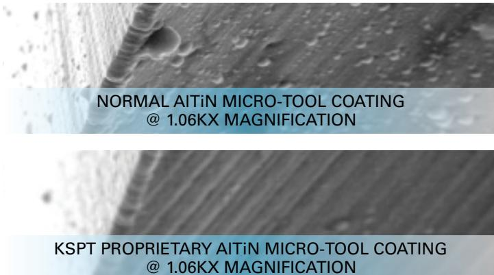
One common misconception is that coated micro tools are often unnecessary because most machines cannot reach sufficient spindle speed to warrant the additional expense of a coated tool. Our testing shows AlTiN coating increases tool life by 250 percent, even when the cutting speed is well below that recommended for uncoated carbide. In other words, coating cost is justifiable, even at low spindle speeds.
